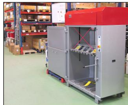
The door of NP80-II can be fully opened (180°), so that the bale can be easily removed even in small spaces.
