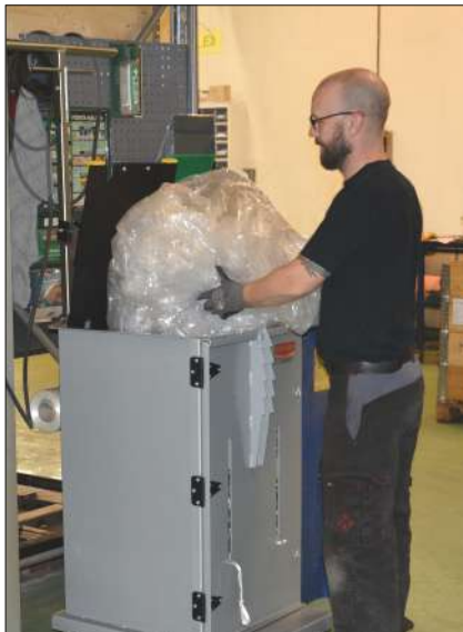
Load the material into the chamber and push the press ram down.
