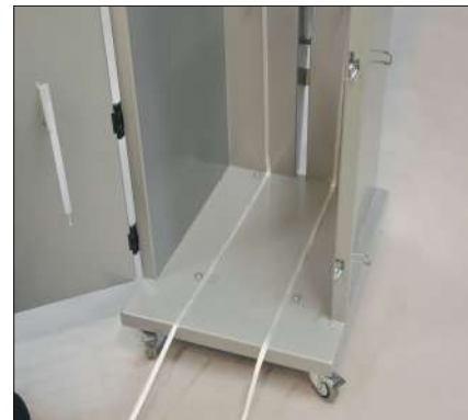
The bale strapping is pulled down along the chamber floor and attached at the front.
