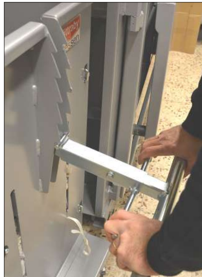
The press ram is automatically locked in its down position, keeping the material under pressure. The press ram is released by a quick hand grip.
